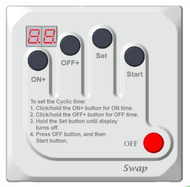
\*\* Once time setting is done simply press the timer Start button whenever you want to run the motor. For any other time just repeat the steps.
